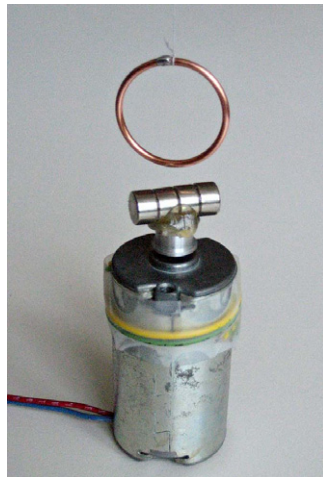
Figure 4. Permanent magnets are glued to a motor. When rotated they produce a rotating magnetic field and rotate the ring.
