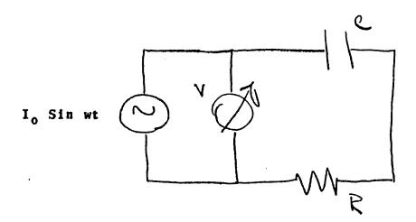
A current generator with negligible internal resistance is connected in series with a capacitor and a resistor. A meter calibrated for x.m.s. voltage is connected across the generator. What value will the voltmeter read if its impedance is much larger than that of any of the other elements in the circuit?
