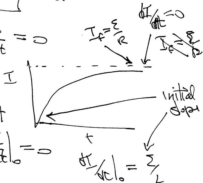
If we have a current I and remove the battery at  $t=0$ :
