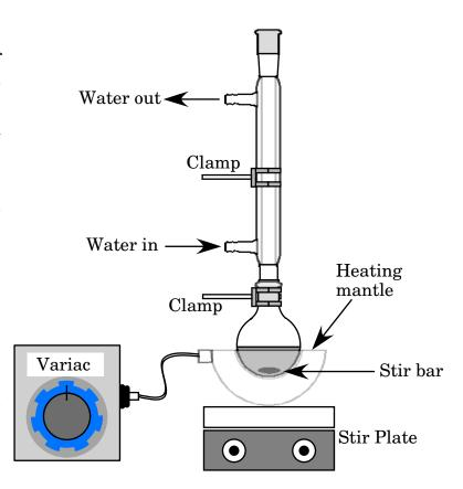
stirring. It is normal for some of the stilbene to precipitate; the precipitated stilbene should redissolve during the reaction. Add 0.8 mL 30% hydrogen peroxide in dropwise fashion. The solution should become dark yellow as the hydrogen peroxide is added. Continue refluxing until the reaction mixture is a cloudy white in appearance (about 20 minutes).
