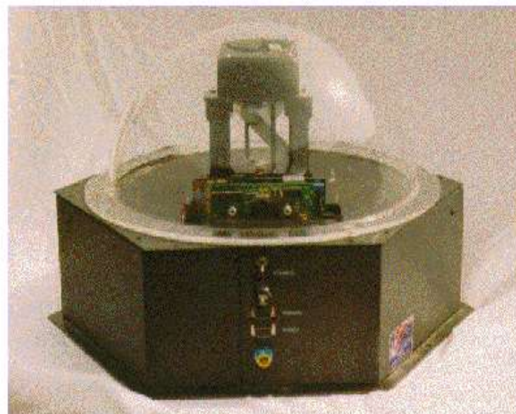
Figure 6.15: Denning Branch International Robotics (DBIR) can see active targets at up to 183 meters (600 ft) away. It can identify up to 32 active or passive targets. (Courtesy of Denning Branch International Robotics.)
