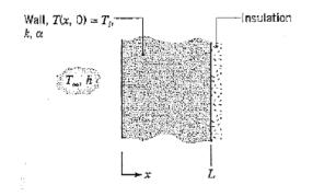
For a particular wall, case 1, the temperature at  $x=L_1$  after  $t_1 = 100$  s is  $T_1(L_1, t_1) = 315$ °C. Another wall, case 2, has different thickness and thermal conditions as shown below.
