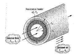
Liquid pumped through the tube is at a temperature  $T_{\infty,i}$ and provides a convection coefficient  $h_1$  at the inner surface of the composite. The outer surface is exposed to ambient air, which is at  $T_{\infty,o}$  and provides a convection coefficient of  $h_o \bullet$  Under steady-state conditions, a uniform heat flux of  $q_h$ " is dissipated by the heater.
