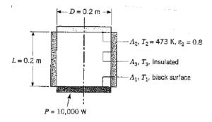
Determine the operating temperature of the lower plate  $T_1$  and the temperature of the insulated side  $T_3$ .
