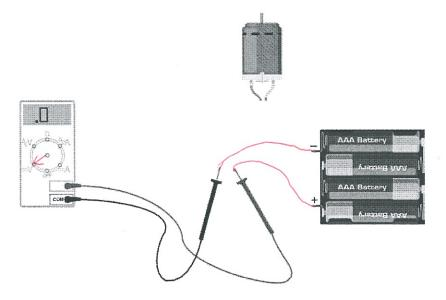
b.) On the diagram below set the knob on the DMM (draw a line from the middle of the circle to one of the outside options) and connect the probes as appropriate to measure the **resistance** of the motor.
