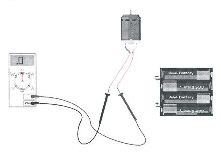
c.) On the diagram below set the knob on the DMM (draw a line from the middle of the circle to one of the outside options) and connect the probes as appropriate to measure the current of the motor.
