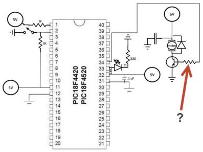
(a) Assuming they measured the motor's resistance as 80 ohms what size resistor should they use for the resistor with the question mark? Show your work, using 6.0 volts for the motor power, and state both the exact resistor size and the real resistor size you'd use. (Select a size from the E6 or E12 series. Hint: we covered this on day 2.)
