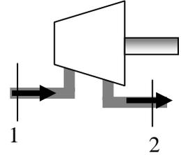
The adiabatic turbine is designed to operate with negligible changes in kinetic energy and gravitational potential energy at steady-state conditions.
