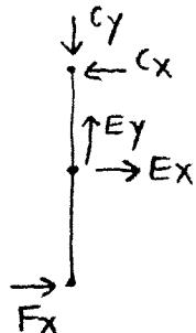
$$\begin{aligned} \textcircled{4} \quad \sum F_x &= 0 & F_x + E_x - C_x &= 0 \\ \textcircled{5} \quad \sum F_y &= 0 & E_y - C_y &= 0 \\ \textcircled{6} \quad \sum \vec{M}_c &= 0 & (F_x)(L_4 + L_5) + (E_x)(L_4) &= 0 \end{aligned}$$
