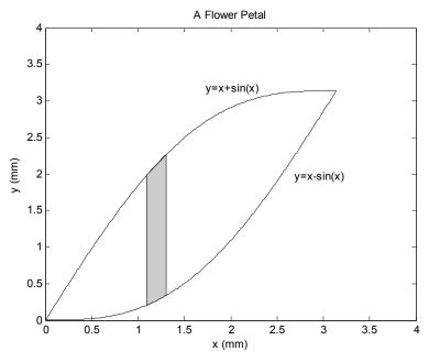
The equation for the y-centroid of the shape may be written (using a vertical strip) as
