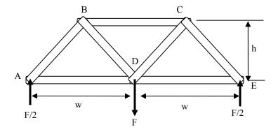
A uniform bar, ABCD, whose cross sectional area is 0.5 in<sup>2</sup> is loaded with the forces shown.
