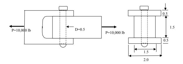
By examining the pin, the yoke, and the bar, find the overall factor of safety for the joint.
