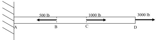
The tensile stress in section BC of the bar is
