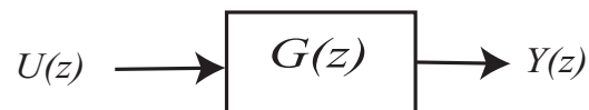
Figure 5: Discrete-time transfer function, G(z) = \frac{Y(z)}{U(z)} . Discrete-time transfer functions are often implemented in terms of the difference equation they represent.
