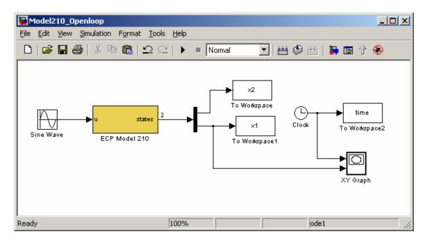
This particular implementation has the input signal in  $\underline{\mathbf{cm}}$  and the position of the two carts measured in  $\underline{\mathbf{cm}}$ . For this implementation, the position of the first cart (x1) is plotted as a function of time as the ECP system runs. (Note that the length of time the XY Graph plots the position of the first cart is hard coded, i.e. it cannot be a variable.)
