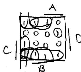
$$A'B'D' + A'C'B' + \underline{AB'C'D'} + BC'D' + \underline{\underline{CD'}}$$
