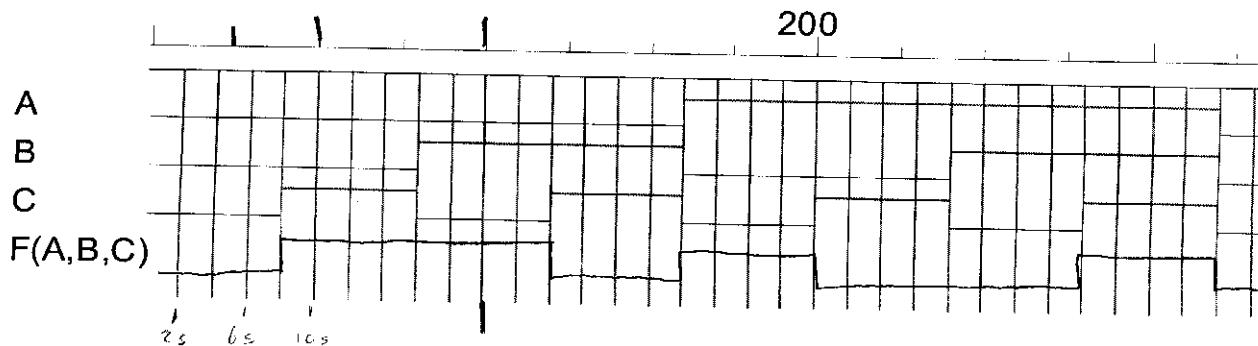
$$T_A = 160 \text{ units} \left( \frac{2 \text{ s}}{10 \text{ units}} \right) = 32 \text{ s}$$
