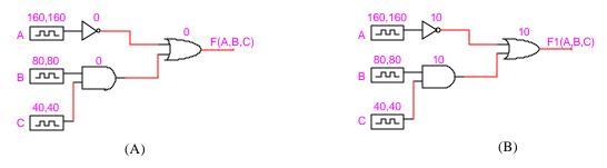
(A) Draw the output waveform of F(A,B,C) with zero time delay gates for all the input combinations. The grid interval is 10 time units.
