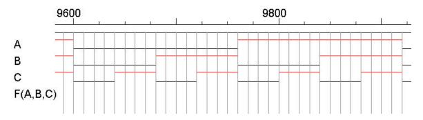
(B) Draw the output waveform of F1(A,B,C) with 10-unit time delay gates for all the input combinations. The grid interval is 10 time units.
