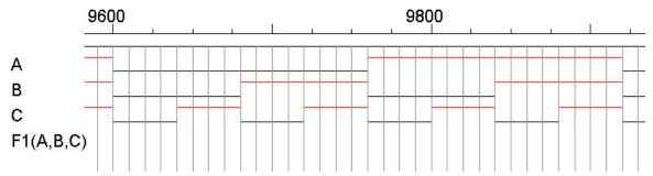
2. Implement and simulate a full adder (addend, augment and carry-in) with standard 74 series of chips. The 74 series of chips are in device library 7400devs.clf that comes with LogicWorks 4. Assuming zero delay, attach a printout of your circuit schematic and waveforms with your homework submission. Verify the truth table on the waveforms by filling in the truth table on the waveforms. (Here are some relevant chips: 74 04 Inverters, 74\_08 AND gates, 74\_32 OR gates.)
