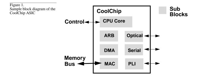
Figure 2. Sample harness block diagram of the CoolChip ASIC
