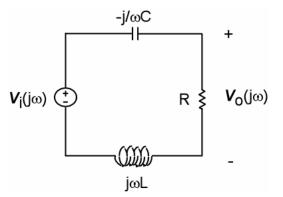
The peak amplitude of the transfer function is 1 at  $w = 1/\sqrt{LC}$ .
