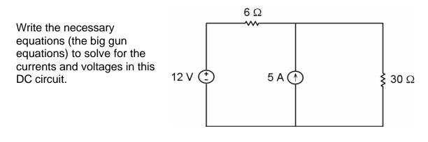
Now, suppose we have solved for the currents and voltages in the above circuit. Find the power delivered by each source. (check your work:  $P_{del (12 V)} = -46 W$ ,  $P_{del (5 A)} = 175 W$ )
