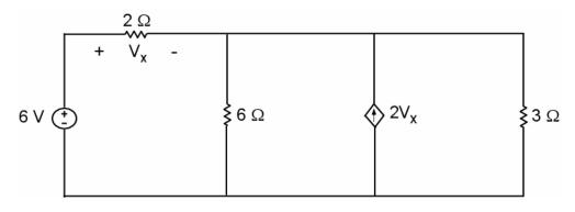
Suppose we've solved for the currents and voltages; find the power absorbed by the  $3\Omega$  resistance. (*Check your work:*  $P_{ab(3 \ W)} = 8.33 \ W$ )
