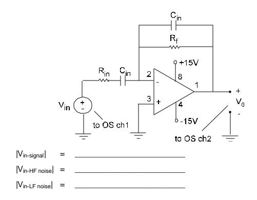
7. At the output, measure the signal amplitude, LF noise amplitude, and HF noise amplitude. (amplitude is ½ of the peak-to-peak values)
