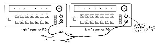
Measure R<sub>in</sub> = \_\_\_\_\_, R<sub>i</sub> = \_\_\_\_\_, and C = \_\_\_\_\_. Use these measured values (DDM for Rs, LCR meter for C) when calculating model predictions and in producing MATLAB-generated plots.
