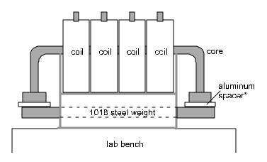
\*Note that aluminum is nonmagnetic—the aluminum spacers act as air gaps.
