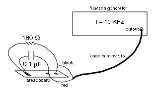
**Important practical information**: The function generator is not an ideal voltage source—it has an internal resistance of 50  $\Omega$ . Also, the capacitor is not an ideal capacitance—it has some dielectric losses (at these frequencies R<sub>c</sub> should be very large). Therefore, a more accurate model for the circuit would be
