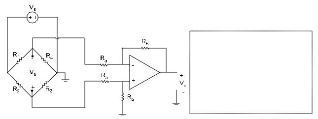
ii) A filtering stage is needed. Design an active *lowpass* filtering stage to filter V<sub>0</sub> with  $\omega_b$ =1000 r/s and a gain of 20dB. Use C = 0.01mF Neatly add this stage to the above schematic.
