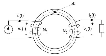
The voltage induced in the coil is  $v_2(t)$ , which is given by:
