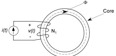
The MAGNETOMOTIVE FORCE (MMF), *F*, pushes the flux around and is analogous to voltage in an electrical circuit. The units of MMF are ampere-turns, and  $\mathscr{F} = N_1 i$ .
