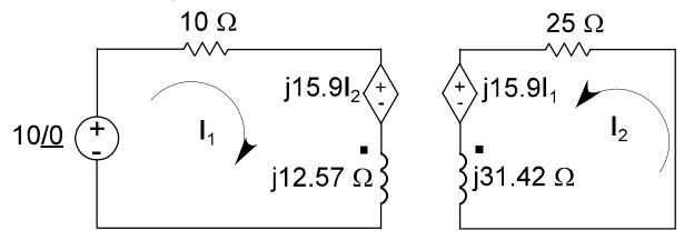
The mesh equations are:  $-10/0+(10 + j12.57)I_1 + j15.91I_2 = 0$  $j15.91I_1 + (25 + j31.42)I_2 = 0$
