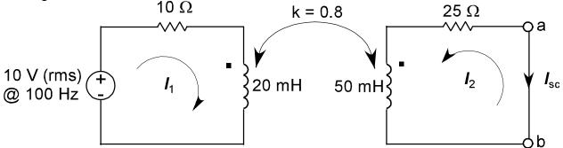
We have to start by getting the equivalent circuit, this means determining M.
