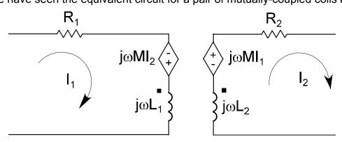
An ideal transformer has no losses, so both R's are zero, k = 1.0, and the core reluctance is zero, meaning the inductances are infinite. Applying Thevenin to Norton conversions gives:
