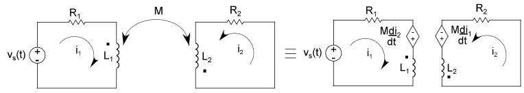
Once again, the magnitude of the mutual voltage is always the mutual inductance times the rate of change of the current in the other coil. In the above circuit,  $i_1$  enters at its dotted end; therefore the mutual voltage in mesh 2 has its "+" at the **bottom** because coil 2's dot is at the **bottom**. Since  $i_2$  enters at its non-dotted end the mutual voltage in mesh 1 has its "+" at the **bottom** because coil 1's dot is at the **bottom**.
