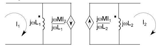
Consider the left-hand side;  $j_{\omega}L_1$  is an open-circuit because  $L_1$  is infinite. The  $j_{\omega}$  terms in the current source cancel and we have M divided by  $L_1$ , which gives:
