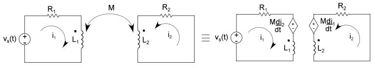
Notice that the magnitude of the mutual voltage is always the mutual inductance times the rate of change of the current in the other coil. In the above circuit, both currents enter the coils at the dotted end; therefore, both mutual voltages have their "+" signs at the **top** because the coils have their dots at the **top**.
