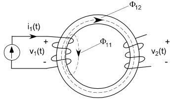
$\Phi = \Phi_{11} + \Phi_{12}$  is the total flux produced by the MMF in coil 1, i.e.  $\Phi = N_1 i_1(t)$  $\Phi_{12}$  is the "main flux"  $\Phi_{11}$  is the "leakage flux"
