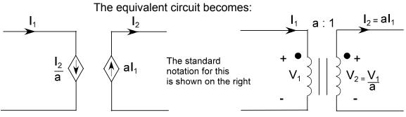
The two bars in between the coil symbols mean that the transformer is wound on a ferro-magnetic core. If these were not present, then the transformer would be "air-cored".
