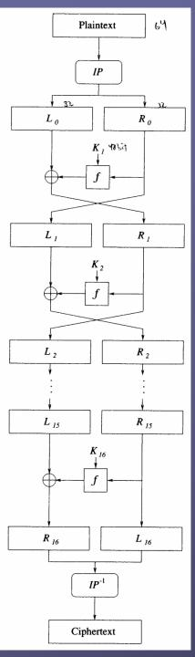
DES has the same structure as EDEN except it uses initial permutations (IP)
