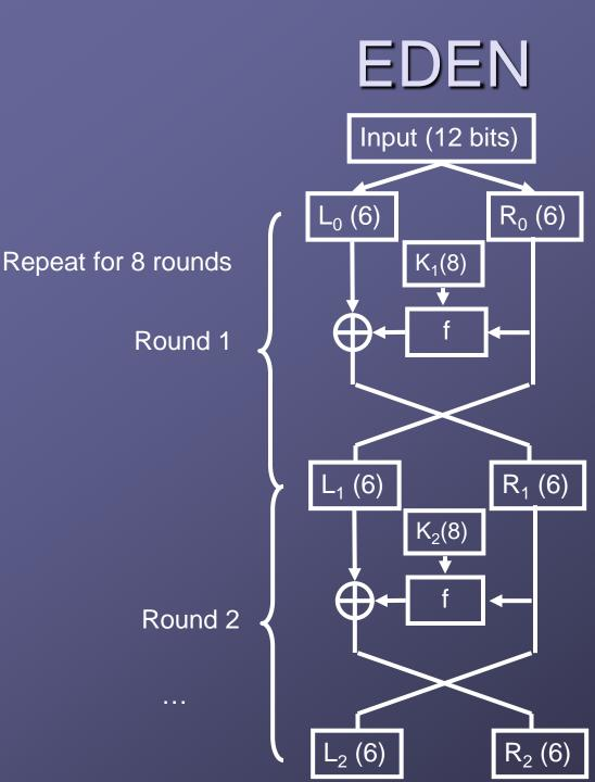
The key, K<sub>i</sub> for round i is derived from a 9-bit key K.
