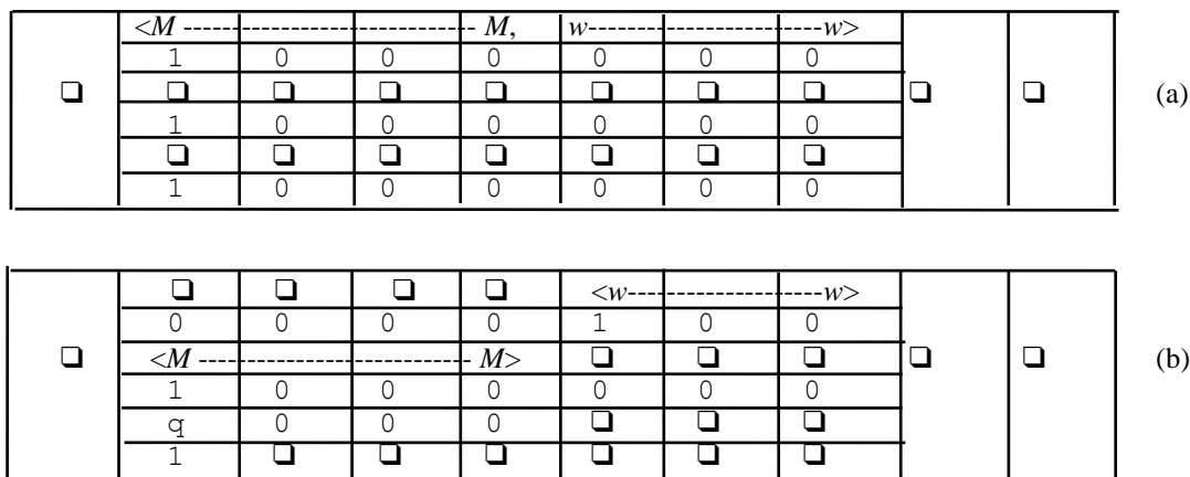
Figure 17.10 The tapes of the universal Turing machine U
