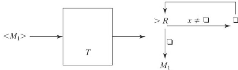
The machine  $M_2$  (output of  $T$ ) empties its tape, then runs  $M_1$ .
