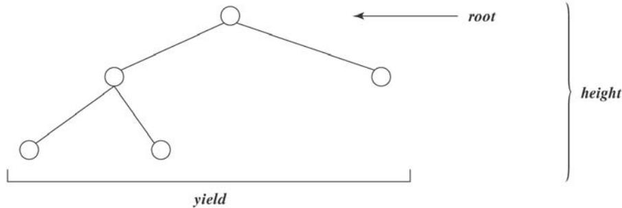
**Theorem:** The length of the **yield** (concatenation of leaf nodes) of any tree  $T$  with height  $h$  and branching factor  $b$  is  $\leq b^h$ .
