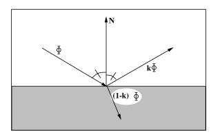
Figure 4.3: Reflection from an ideal specular surface.
