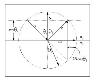
Figure 2.2: Geometry for light hitting a smooth surface.
