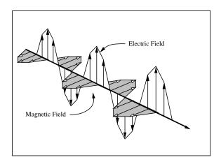
Figure 2.1: Propagation of an electromagnetic wave
