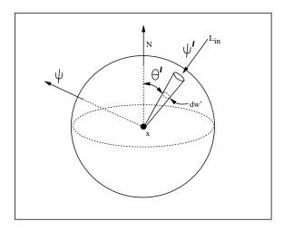
Figure 3.8: Geometry for Directional Rendering Equation.
