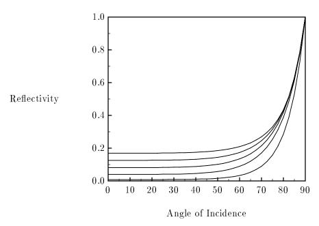
**Figure 2.3**: Reflectivity of light passing from air to dielectrics of various indices of refraction (1.2, 1.5, 1.8, 2.1, 2.4 bottom to top). Curves were generated directly from Fresnel Equations.
