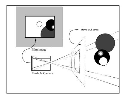
Figure 1.3: A pin-hole camera model of image acquisition.
