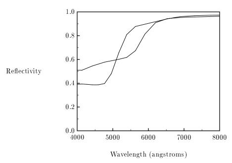
Figure 2.6: Normal incidence reflectivity for various wavelengths for gold (bottom curve at y-axis) and copper. Curves were generated directly from Fresnel Equations using data from Palik [82].
