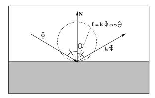
Figure 4.5: Diagram of energy reflection from combined surface.
