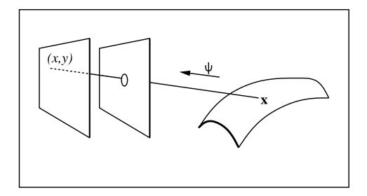
**Figure 5.4**: The image function at (x, y) is the radiance at **x** traveling toward the pin-hole.
