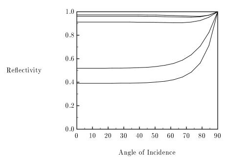
**Figure 2.9**: Reflectivity of gold for wavelengths 4000, 5000, 6000 7000, and 8000 angstroms (bottom to top). Curves were generated directly from Fresnel Equations using data from Palik [82].
