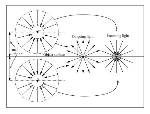
Figure 3.6: Incoming and outgoing radiance distributions at the surface are constructed from piecing together functions on either side of the surface.
