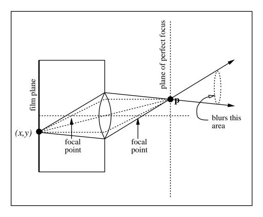
Figure 5.2: A thin lens camera
