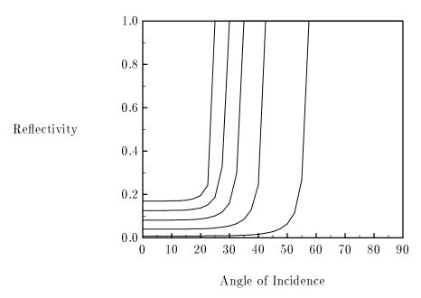
**Figure 2.4**: Reflectivity of light passing from dielectrics of various indices of refraction (1.2, 1.5, 1.8, 2.1, 2.4 bottom to top) to air. Curves were generated directly from Fresnel Equations.
