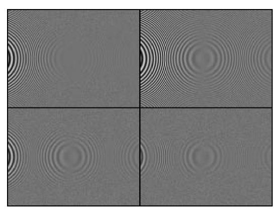
**Figure 5.1**: Images generated by (left to right, top to bottom) nonuniform filter, box filters with one pixel width, two pixel width, and three pixel width. The circular pattern on the left of each image is correct, while the circular pattern centered in the middle and on the right are caused by aliasing.
