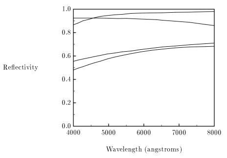
Figure 2.7: Normal incidence reflectivity for various wavelengths for (bottom to top on y-axis) nickel, platinum, silver, and aluminum. Curves were generated directly from Fresnel Equations using data from Palik [82].
