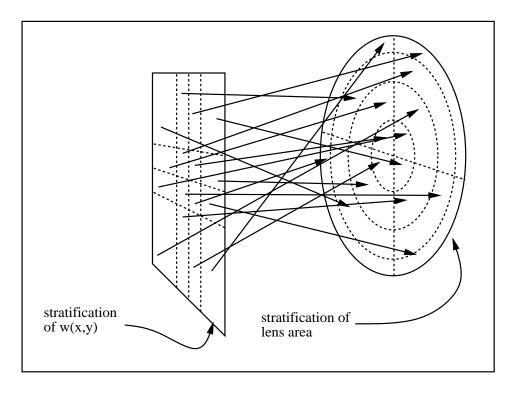
Figure 5.7: 16 rays fired from all strata of pixel toward 16 strata on lens
