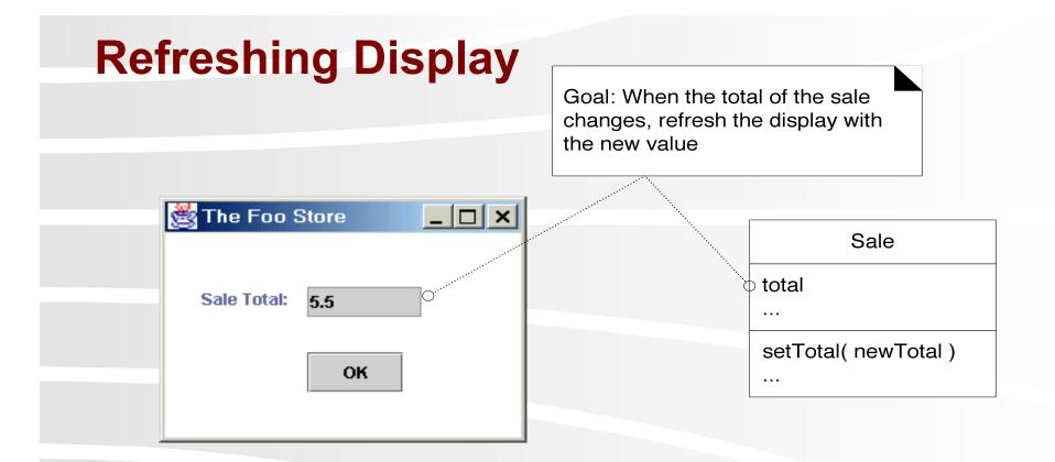
How do we refresh the GUI display when the domain layer changes without coupling the domain layer back to the UI layer?
