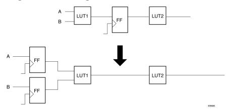
Backward Register Balancing moves a flip-flop at the output of a LUT to a set of flip-flops at its inputs.
