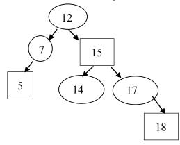
b) [4 points] Remove the following element: 7 from the *Red-Black* tree below. Use top-down removal and show intermediate trees in case of rotations. Indicate which nodes are red and which ones are black. In the tree below, red nodes are drawn as a square.
