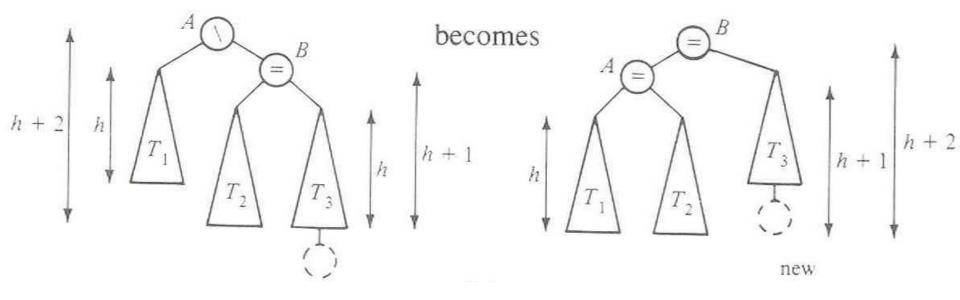
We rotate by pulling the "too tall" sub-tree up and pushing the "too short" sub-tree down
