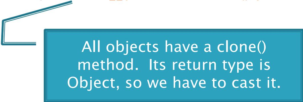
All objects have a `clone()` method. Its return type is `Object`, so we have to cast it.
