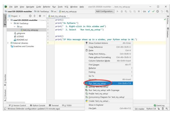
If a sub-window shows up with the output from the **print** statements (as shown to the right), your Python has been set up correctly!
