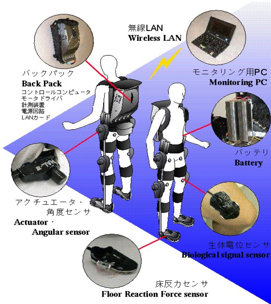
The HAL 3 system assists the user in walking. Image source: http://www.cyberdyne.jp/ENG/hal.html
