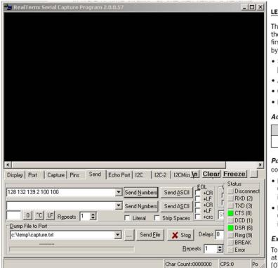
This command controls the LEDs on Create. The state of the Play and Advance LEDs is specified by two bits in the first data byte. The power LED is specified by two data bytes: one for the color and the other for the intensity.
