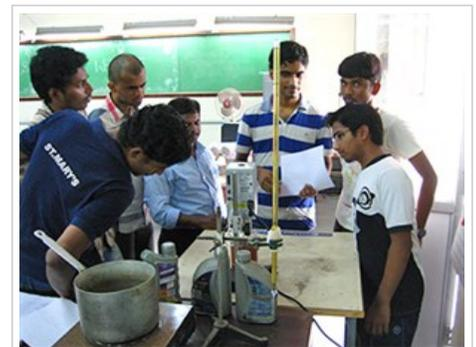
Students test the viscosity of motor oil in a laboratory at IIT Madras.
