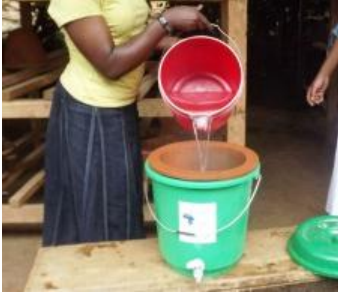
Visual 3 The ceramic filter in Visual 2 in use
