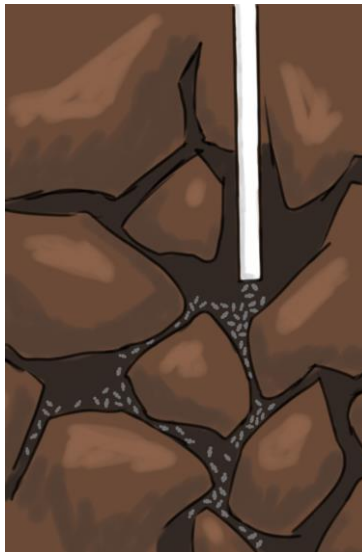
Figure 2: The carbon dioxide is transported down a pipeline and stored in a geological formation. The liquid carbon dioxide fills in the gaps in the porous rocks and over time will turn into chalk, a stable form of carbon dioxide.
