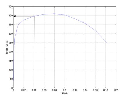
1. Calculate the modulus of elasticity of the material. (Units GPa)
