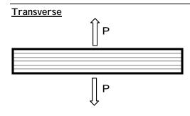
Equal Load in matrix and fiber, similar to two springs in series. The less stiff spring (matrix) provides the most deflection, therefore controls response.
