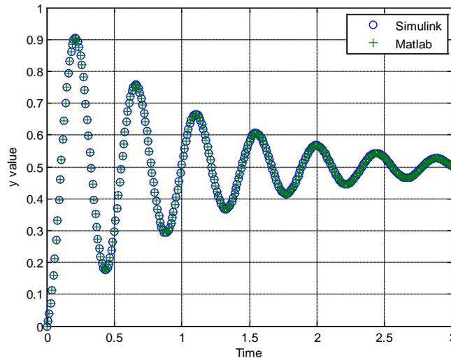
**Figure 1.** Open loop response of the system.
