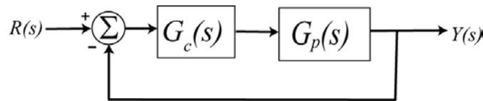
One way to choose the controller is to try and make your closed loop system match a transfer function that you choose (hence the name model matching). Let's assume that our **desired** closed loop transfer function,  $G_o(s)$ , our plant can be written in terms of numerators and denominators as
