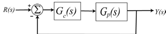
a) Using the results from problem 4, determine the controller so that the closed loop system matches a second order ITAE (Integral of Time and Absolute Error) optimal system, i.e., so that the closed loop transfer function is
