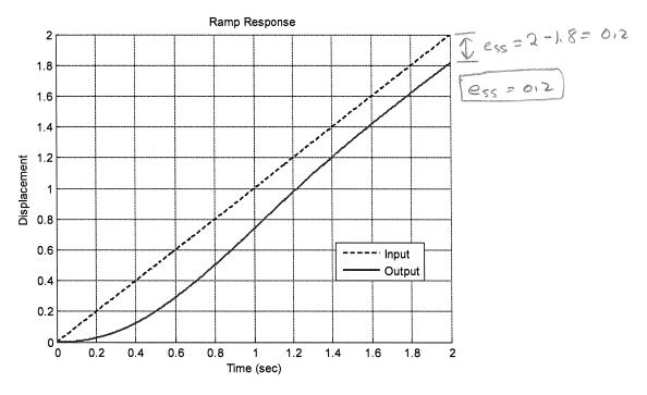
8) Estimate the steady state error for the ramp response of the system shown below:
