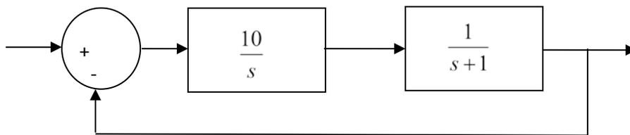
a) If the input to the system is  $r(t) = 8u(t)$ , what is the steady state output?
