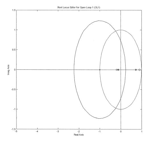
7) With the closed loop pole locations shown in the figure, is the closed loop system stable?
