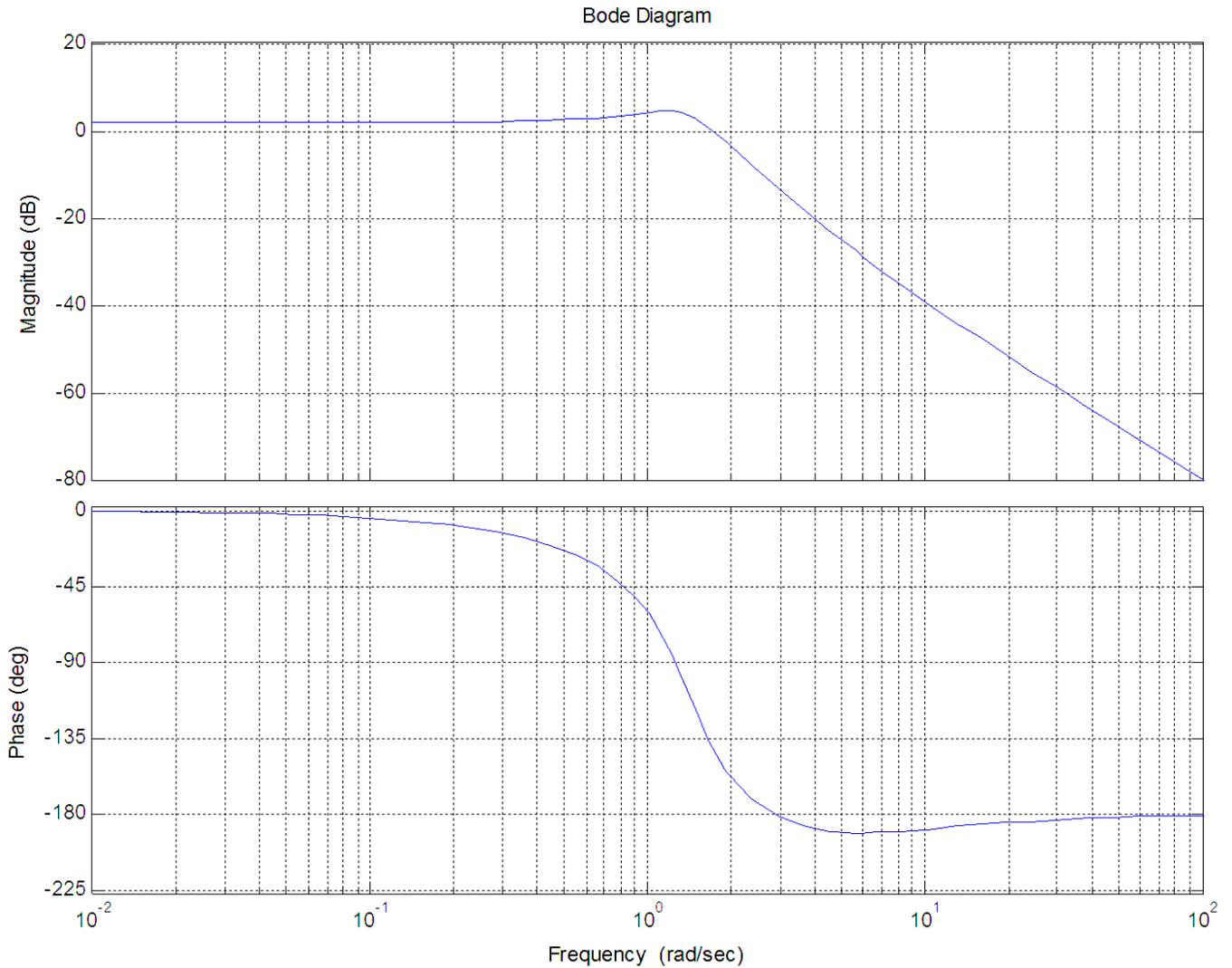
7) The *gain crossover frequency* used to determine the *phase margin* for this system is best estimated as
