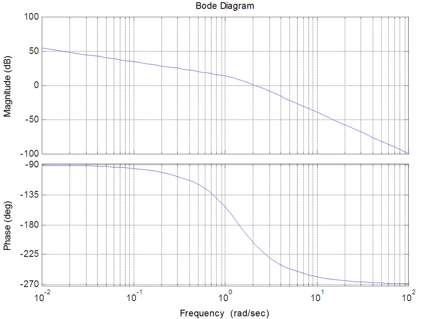
11) The *gain crossover frequency* used to determine the *phase margin* for this system is best estimated as
