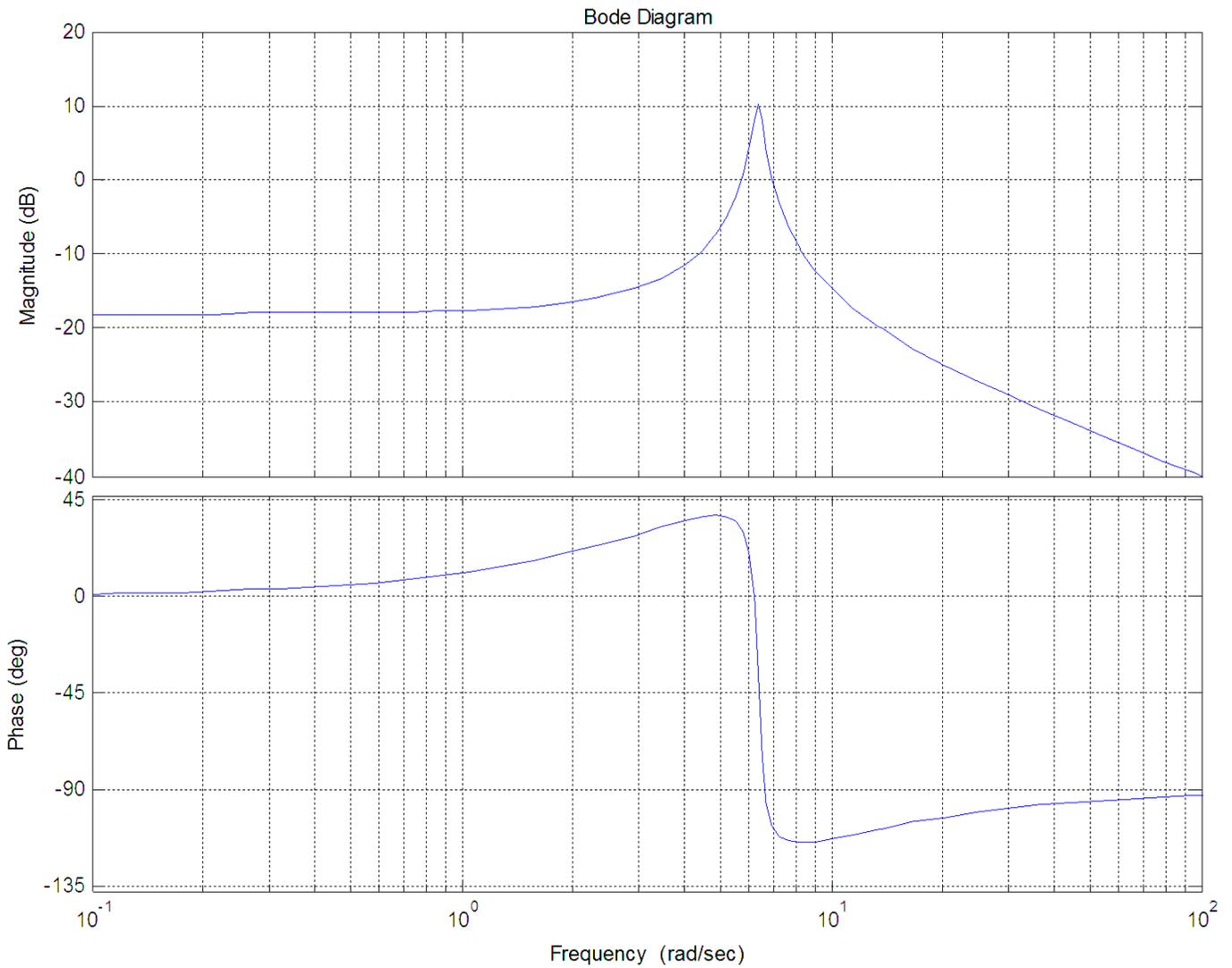
15) The *gain crossover frequency* used to determine the *phase margin* for this system is best estimated as
