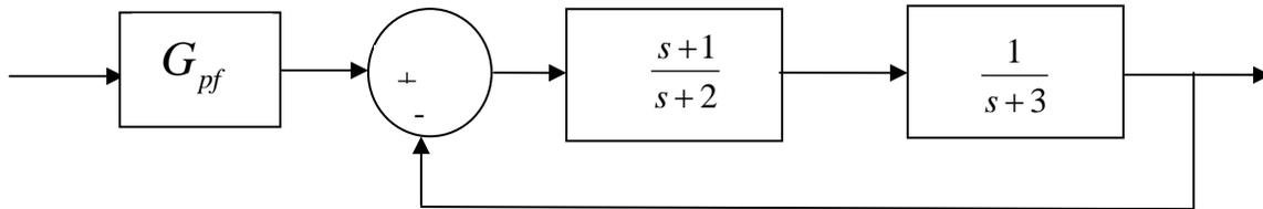
If we want to use a dynamic prefilter to **cancel the closed loop zero** and produce a **zero steady state error for a unit step**, we should choose the prefilter as
