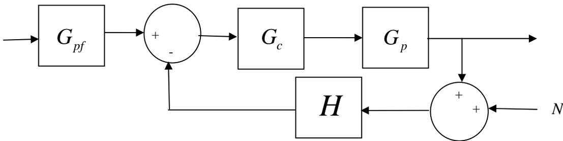
to reduce the effects of sensor noise  $N$  on the closed loop system, we should
